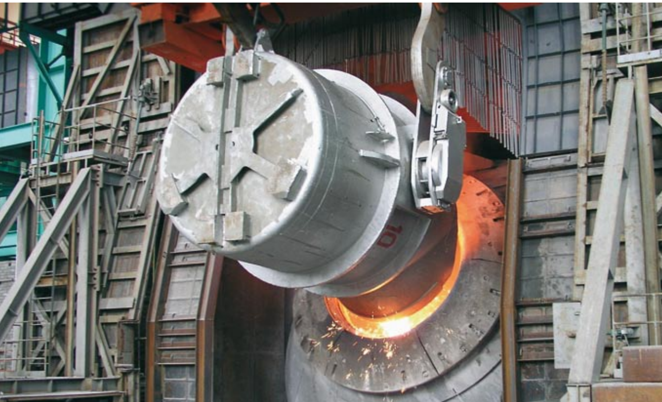
1st hot metal charging at Jiangsu Shagang, Zhangjiagang, China
