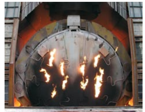
Bottom injection of inert gas for best performance and a long life
